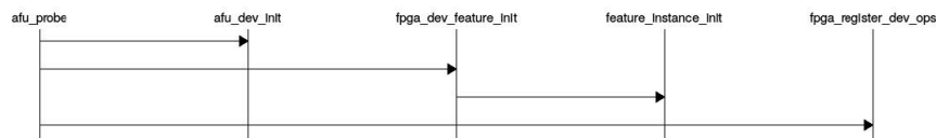
Figure 5. Port Initialization Flow
