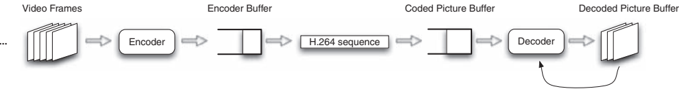
Figure 8.6 H.264 encoder and decoder buffers
