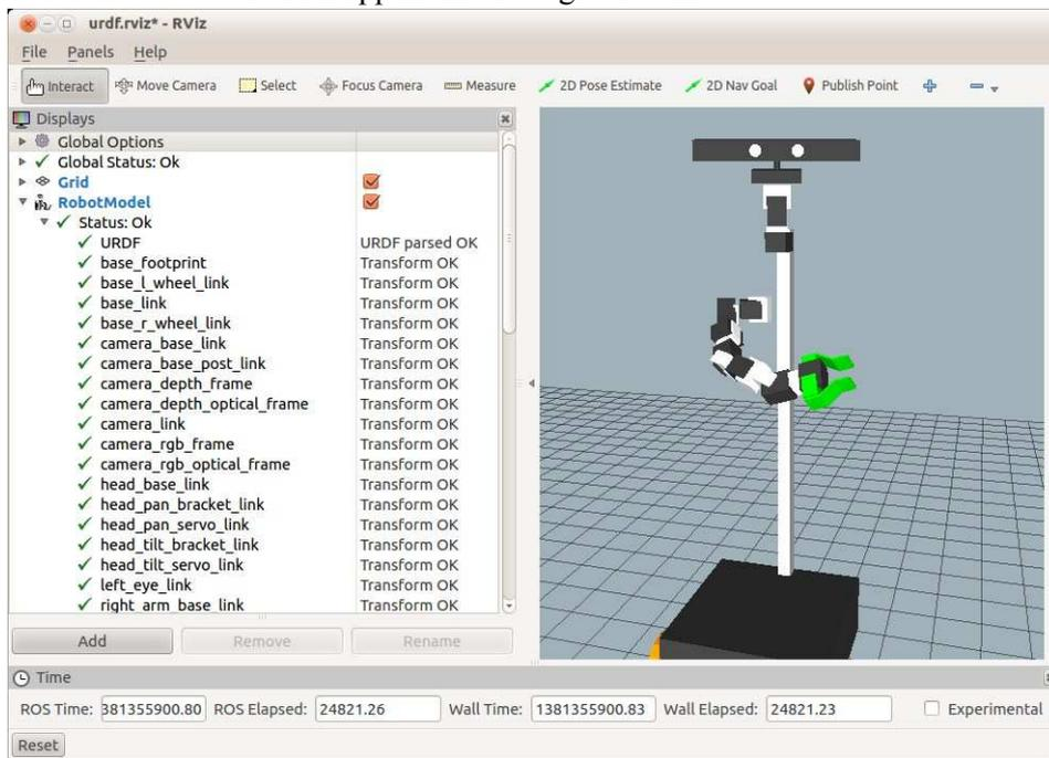
Here we have positioned the joints of the arm as well as the gripper using the slider controls in the joint state GUI.
