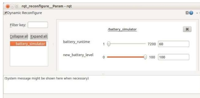
Use the sliders or text boxes to change the battery runtime or battery level.
