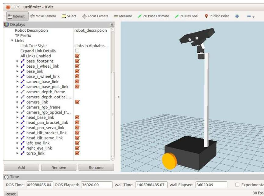
In the meantime, the Joint State Publisher window will now include two new slider controls for the pan and tilt joints as shown on the right. For the image above, the controls were used to pan the head to the left and tilt it downward. With the **Links** sub-menu expanded under the **RobotModel** display, we can see the links that make up the brackets and servos of the pan-and-tilt head.
