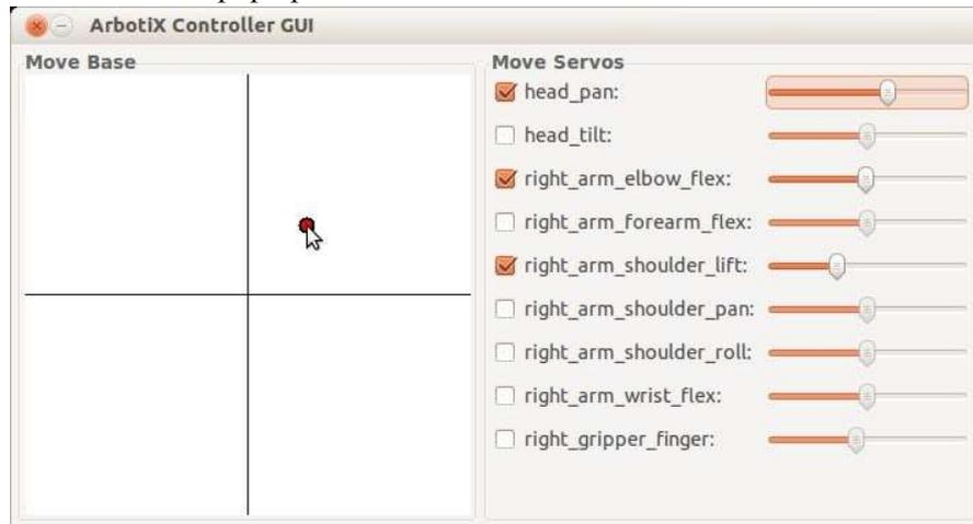
Use the simulated track pad on the left to drive the robot around in `RViz` by grabbing the little red dot and dragging it around. (If the robot does not appear to move, doublecheck that you have set the **Fixed Frame** to `/odom` under the **Global Options** category in `RViz`.) To move a joint, click the checkbox beside a servo name then use the slide control to rotate it.
