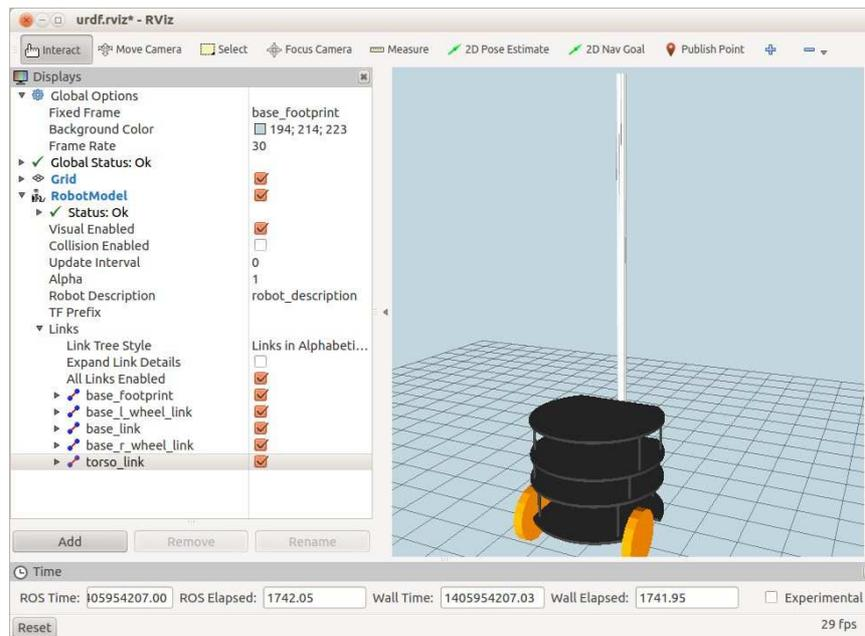
(Remember to toggle the checkbox beside the **RobotModel** display if RViz is still showing a previously loaded model.)
