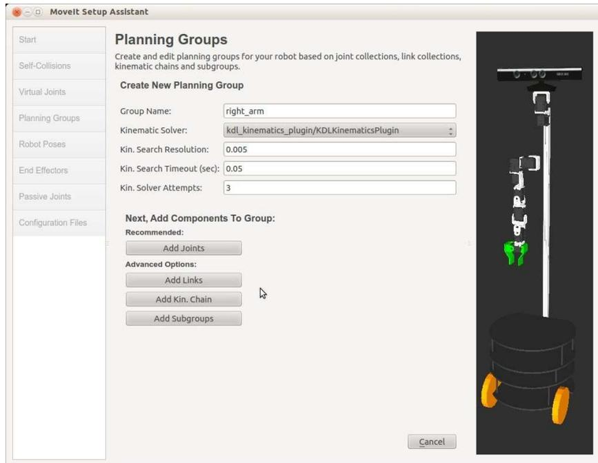
We will add the arm's joints to the planning group as a serial kinematic chain as this is required when using the KDL plugin. Therefore, click the **Add Kin. Chain** button. The next screen should look like the following:
