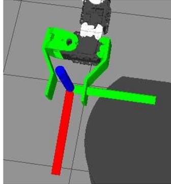
The red, green and blue axes are centered at the desired grasping point and are oriented with the red x-axis parallel to the fingers, the blue z-axis pointing upward from the plane of the gripper, and the green y-axis pointing to the gripper's left.
