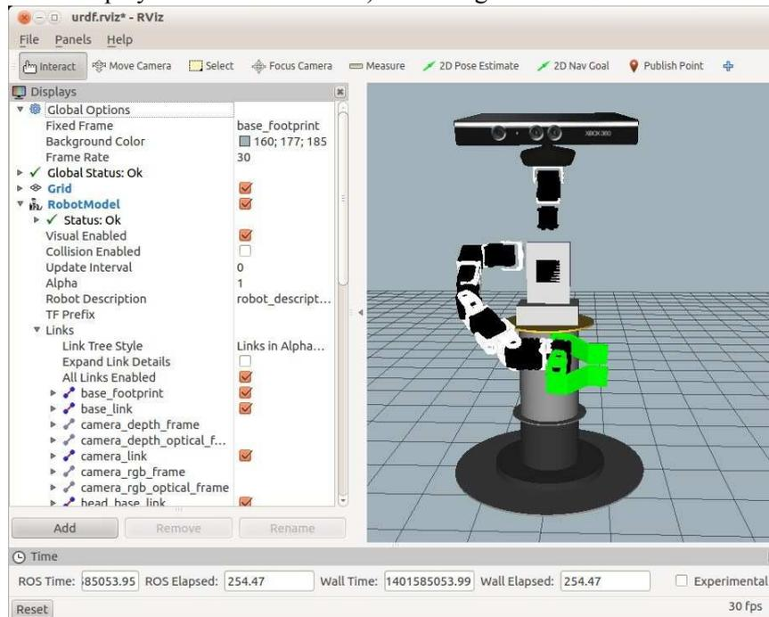
It is instructive to note that the very same URDF/Xacro files for the arm and gripper are used with this "Pedestal Pi" model as with the mobile version of Pi Robot. We are simply attaching the arm and gripper to different base models for the two robots.
