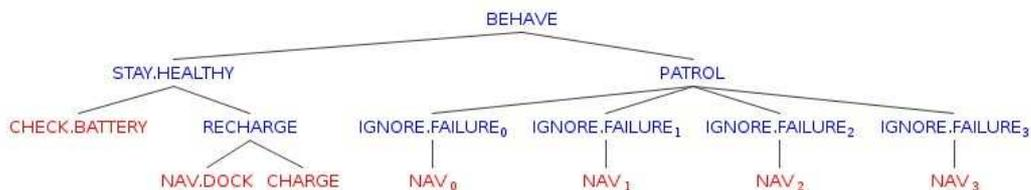
Another way to iterate over a sequence of behaviors while ignoring failures is to simply define a new type of sequence with the ignore failure property built in. The `pi_trees` library includes the `Iterator` composite behavior that does just that.
