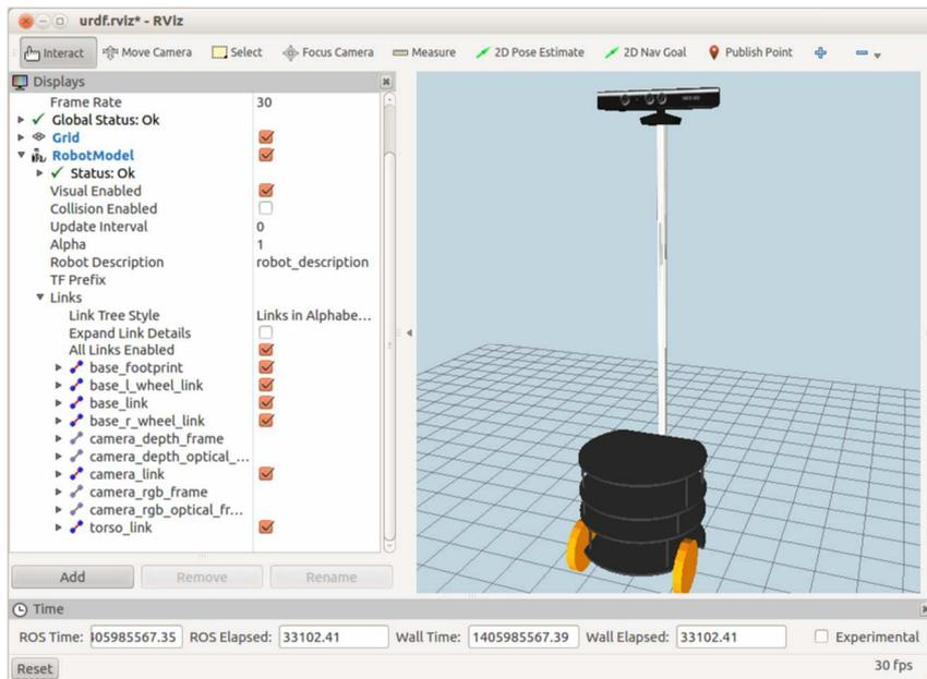
And here is closer view of the mesh including the coordinate axes for the depth and RGB camera frames:
