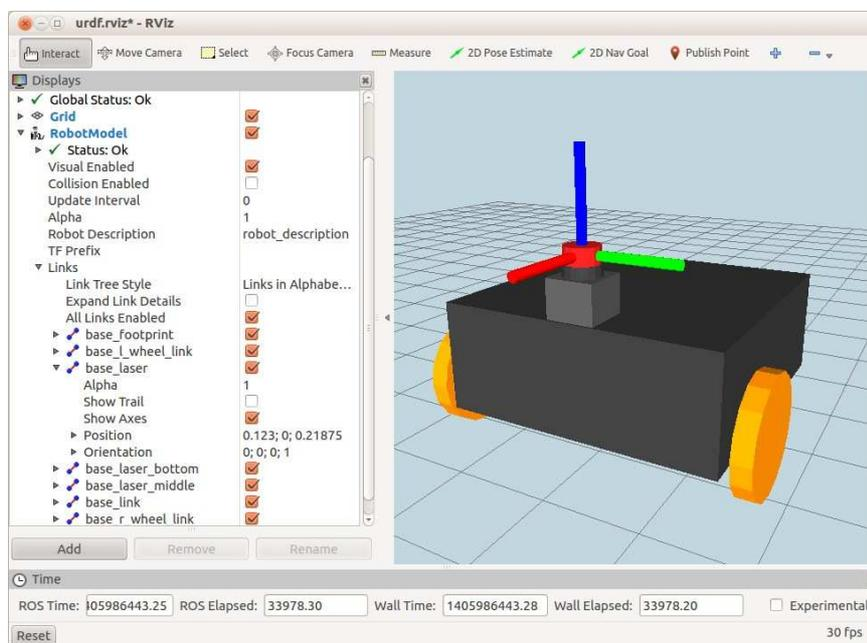
In the image above, we have checked the **Show Axes** checkbox for the `base_laser` link. This allows us to see that the base laser frame is located in the middle of the upper cylinder and that the axes are oriented in the same direction as the base. (Remember that the red axis is in the  $x$ -direction and that we want it pointing forward.)
