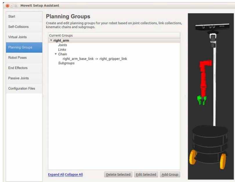
The last link in the chain is often referred to as the "tip" and typically corresponds to the end-effector. Note how in this case, we are using the virtual `right_gripper_link` that was created in the URDF in between the two gripper fingers to make it easier to specify a desired pose for the end-effector.
