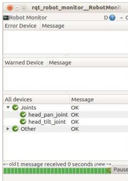
If the USB2Dynamixel controller has successfully connected to the two servos, the two joints will appear in the `rqt_robot_monitor` window as shown above. We will explore this monitor in detail in the next chapter on ROS Diagnostics.
