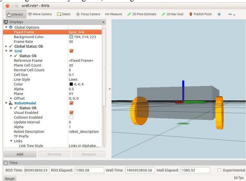
Note how the origin of a URDF box component is placed at the center of the box; i.e. at a height of `base_size_z/2` meters above the bottom of the robot. Consequently, the fixed joint between the `/base_footprint` frame (which rests on the ground) and the `/base_link` frame must include a translation in the z-direction a distance of `base_size_z/2` meters just to get the bottom of the robot up to the ground plane.
