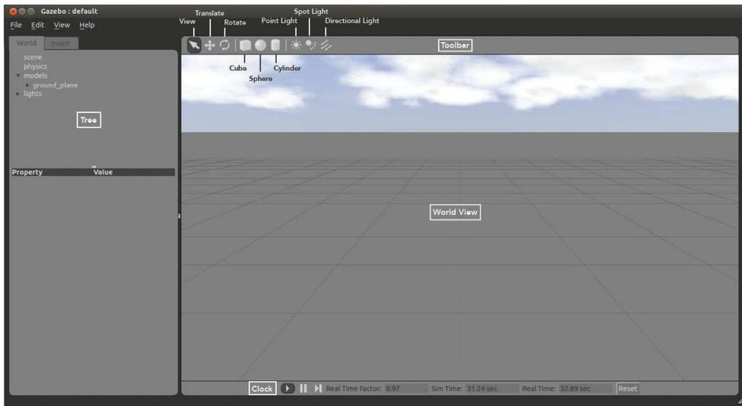
One of the more frequently used menu items is the **Reset Model Poses** command found under the **Edit** menu. This will return the robot and any objects to the poses they had when the simulation was first started. The **Reset World** menu item does the same thing but also resets the clock.
