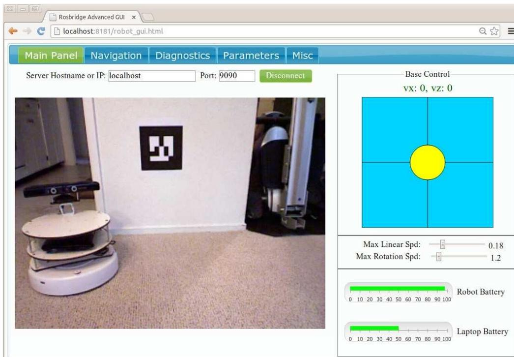
The tabs are arranged across the top—click or tap a tab label to switch to the corresponding screen. Only the **Main**, **Navigation** and **Misc** tabs currently have any function—the **Diagnostics** and **Parameters** tabs are just place holders to serve as additional examples. These tabs are created using the [jqWidgets](#) toolkit and the code can be found in the `robot_gui.html` file.
