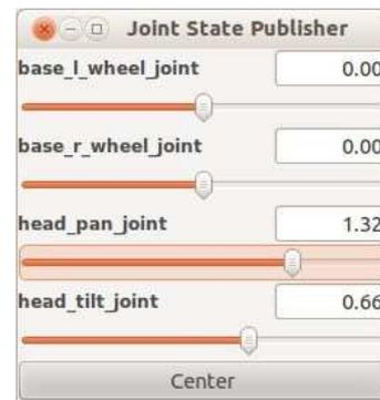
**NOTE:** Recall that ROS uses the right-hand rule for coordinate frames and rotations with the base frame oriented with the x-axis pointing forward, the y-axis pointing to the left, and the z-axis pointing straight up.
