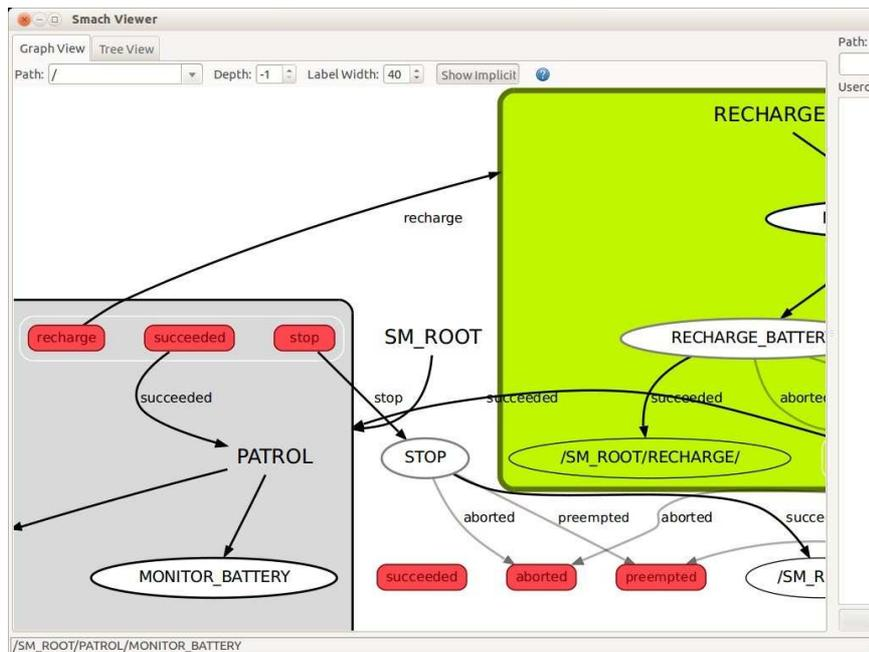
The arcing arrow from the red `recharge` outcome on the left to the green `RECHARGE` box on the right indicates the transition from the concurrence container to the `RECHARGE` state machine when the concurrence produces the 'recharge' outcome.
