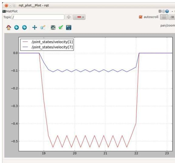
Note how the motions of the two joints begin and end at the same time.
