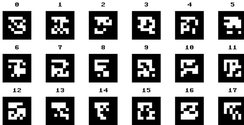
It turns out that certain kinds of checkerboard-like patterns like those shown above are particularly easy to recognize under different lighting conditions, viewing angles, and distances. These patterns are called *fiducial markers* or *AR tags*. AR stands for "augmented reality" because such tags can be added to objects and detected in video recordings so that animations or other artificial labels (such as the name of the object) can be overlaid on the video in place of the tag.
