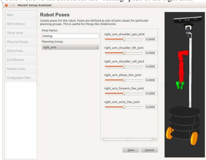
When the arm is positioned the way you want, click the **Save** button. To add another pose, click the **Add Pose** button again. In the following screen shot, we have defined a pose called `straight_forward` with the arm pointing forward and parallel to the floor.
