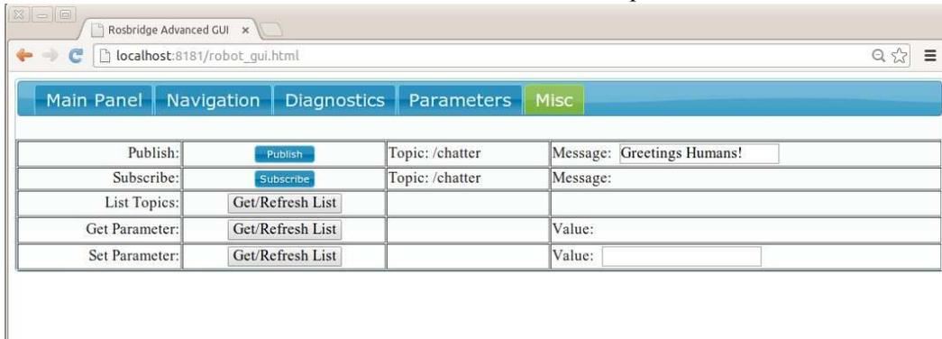
The **Diagnostics** and **Parameters** tabs are currently just place holders defined by the files `tabs/diagnostics.html` and `tabs/parameters.html`. Edit these files to include your own code or remove the tabs altogether by editing the file `robot_gui.html`. For now, the pages simply display the following message:
