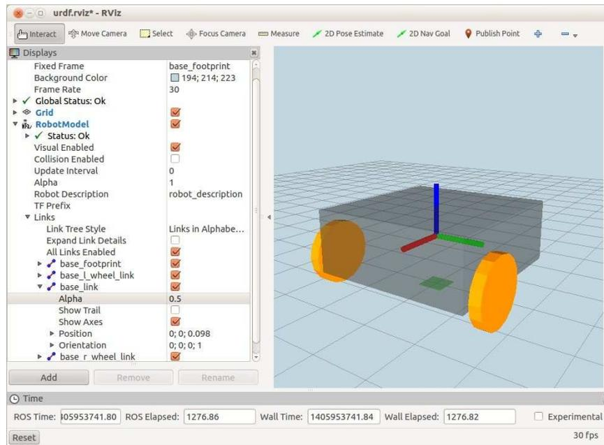
Here we have set the **Alpha** value to 0.5 for the `base_link` and checked the box beside **Show Axes**. RViz always uses the same color code for the frame axes attached to a link: red for the `x`-axis, green for `y` and blue for `z`.
