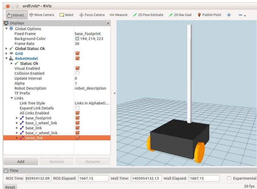
(Remember to toggle the checkbox beside the **RobotModel** display if you are still seeing a previously loaded model.)
