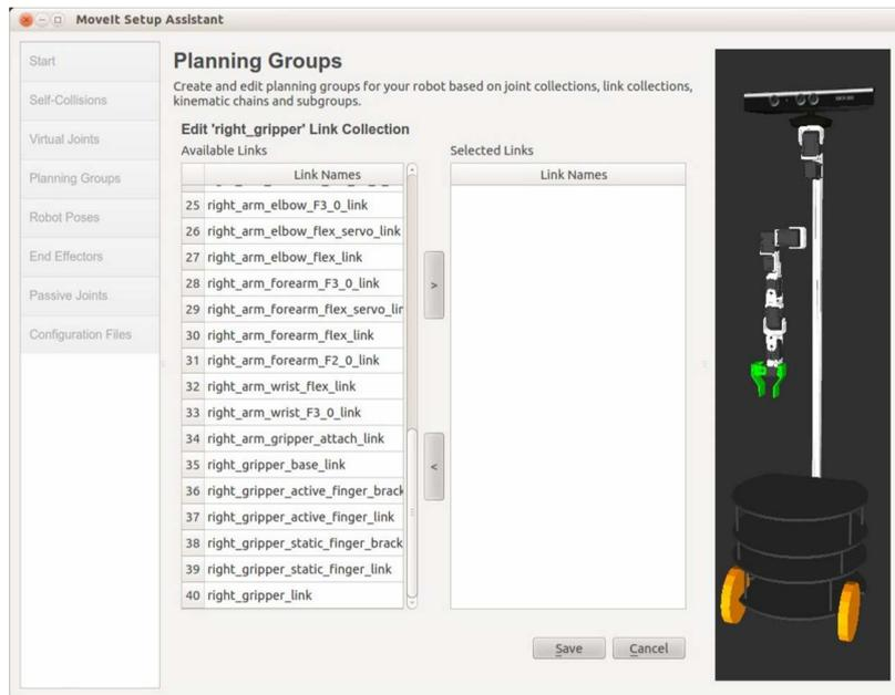
Check that the left and right panels are labeled "Link Names". In the left panel, select all links whose name begins with `right_gripper`, then click the right arrow button to move the links into the right panel. The result should look like this:
