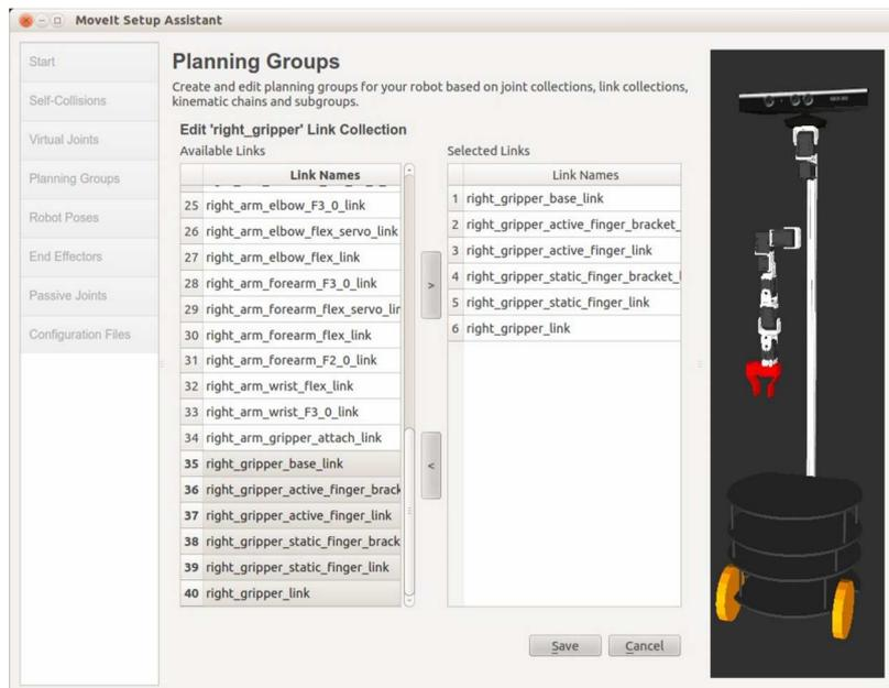
Note how the gripper is now highlighted in red in the image on the right. Finally, click the **Save** button.
