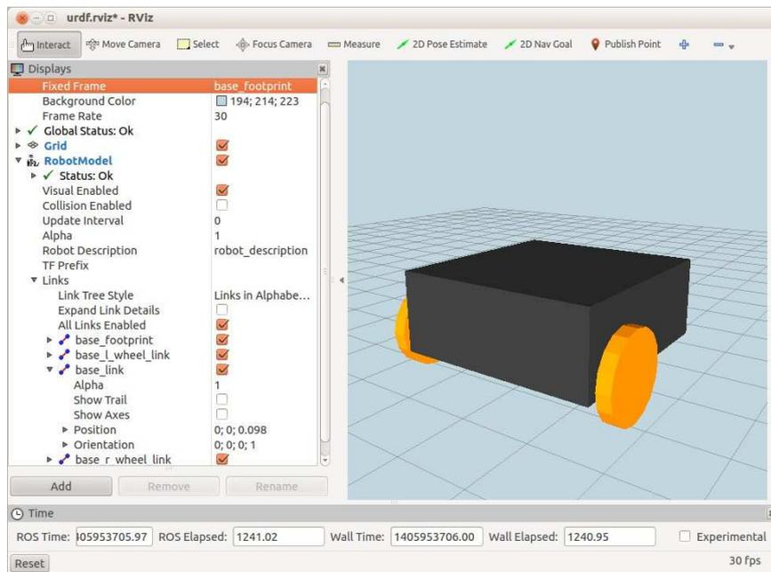
Note how the **Fixed Frame** is set to `/base_footprint`. Keep this in mind as we look at the URDF definition of the base later on.
