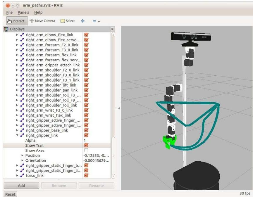
The straight line triangle in the image is formed by the paths taken by the gripper when following the computed Cartesian path. The two curved paths are the trajectories followed when using the regular `go()` command.
