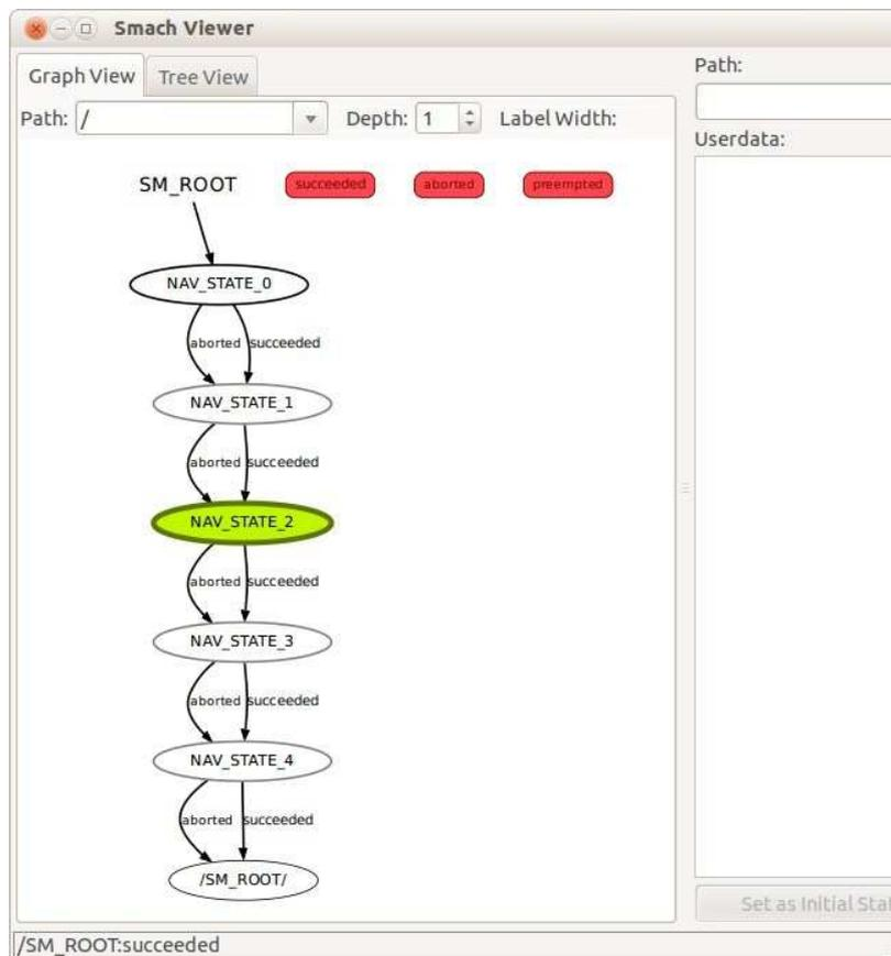
As the robot moves from state to state (i.e. moves from location to location around the square), you should see the appropriate state highlighted in green in the viewer. For a complete description of the SMACH viewer GUI, see the [smach viewer](#) Wiki page.
