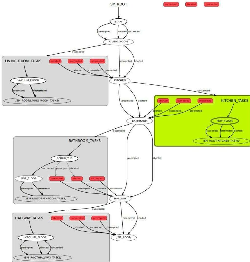
The `clean_house_smach.py` script is fairly straightforward so we'll highlight just the key concepts. The most important concept in the script is the construction of a hierarchical state machine. First, we create a state machine for each room like this:
