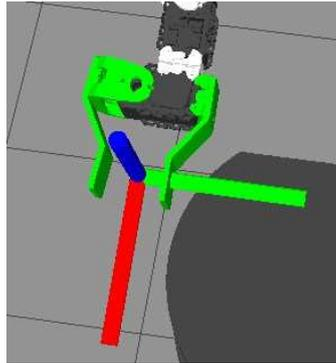
The red, green and blue axes are centered at the desired grasping point and are oriented with the red x-axis parallel to the fingers, the blue z-axis pointing upward from the plane of the gripper, and the green y-axis pointing to the gripper's left.
