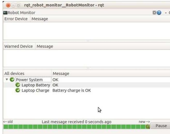
Under the **Power System** category, we have two status messages: one for the battery overall (i.e. it can be detected) and one for the current charge level. The first status is provided by the `laptop_battery.py` node whereas the second is published by our new node `monitor_laptop_charge.py`. Let's take a look at that script now.
