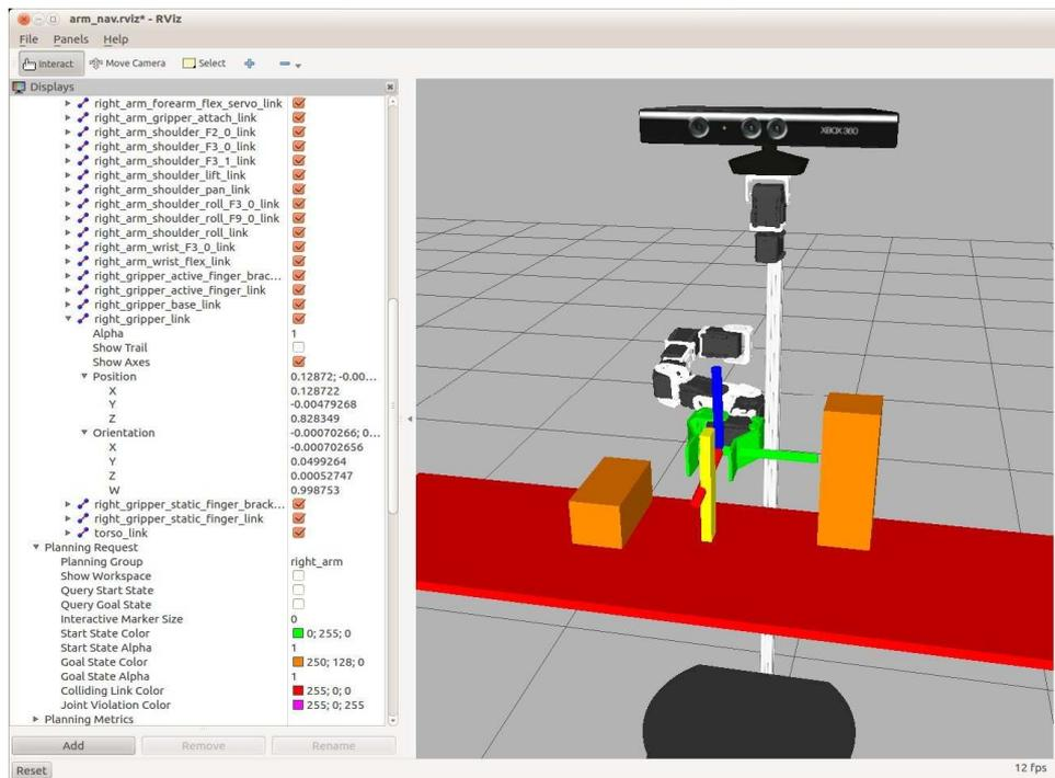
Remember that we defined this frame for planning purposes and placed the axes in between the two finger pads which is where we would typically grasp an object. From the image you can see that we want to align this frame with the target object (the narrow yellow block) and place the origin of the gripper frame near the center of the object.
