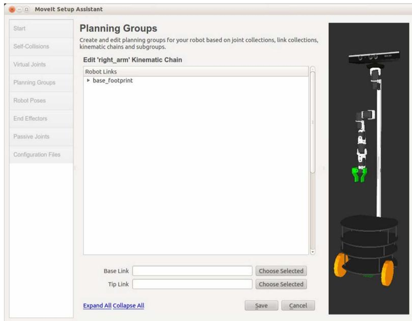
Click the link labeled **Expand All** so see the entire link tree of the robot as shown below. Then select the `right_arm_base_link` in the tree and click the **Choose Selected** button next to the **Base Link** text box. The result should look like this:
