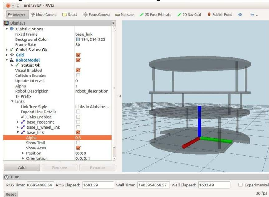
As you can see, this particular mesh defines its origin in the center of the bottom of the base. (Recall that a box or cylinder component has the origin in the middle of the component.) Fortunately the axes are oriented the way we want with the  $x$ -axis pointing in the robot's forward direction.
