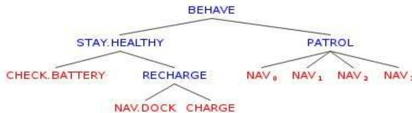
Behavior trees break down complex tasks by branching them into a set of conditions and subtasks. The tree is always executed from top to bottom and left to right. For a given level of the tree, nodes on the left have higher priority than nodes on the right. In the tree shown above, this means that the `STAY_HEALTHY` branch of the tree will always be run before the `PATROL` branch. Similarly, the `CHECK_BATTERY` task will always be executed before the `RECHARGE` behavior.
