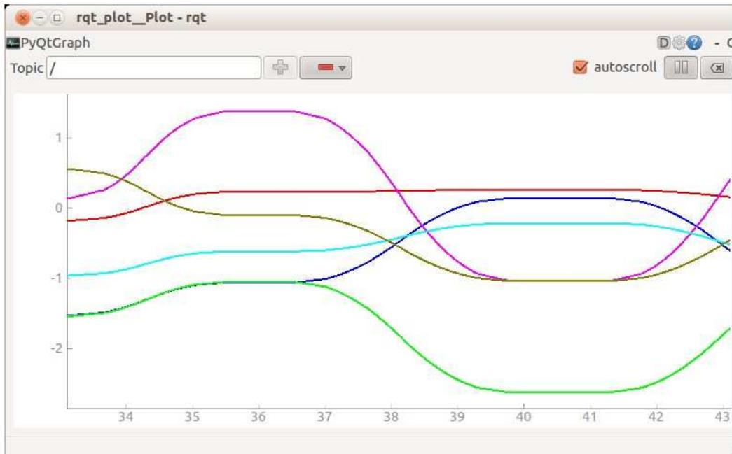
This plot was generated by running `rqt_plot` on the relevant joint positions while the arm was moving. The actual command used was:
