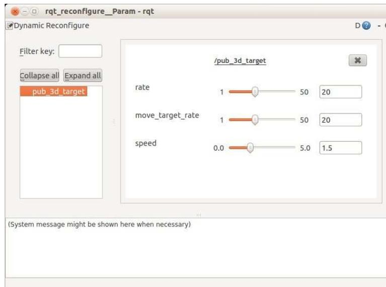
For example, setting the `move_target_rate` to 1 and the `speed` to 2.0 will cause the sphere to jump over larger gaps instead of moving smoothly in between.
