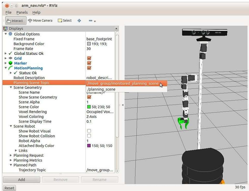
The obstacles initially appear all the same color in RViz which is determined by the setting under the **Motion Planning** display named **Scene Geometry** → **Scene Color** also shown above. Our script sets different colors for individual objects. Real obstacles can be added to the planning scene either from existing knowledge of the robot's environment, or from sensor data such as laser scans and point clouds as we will see later in the chapter.
