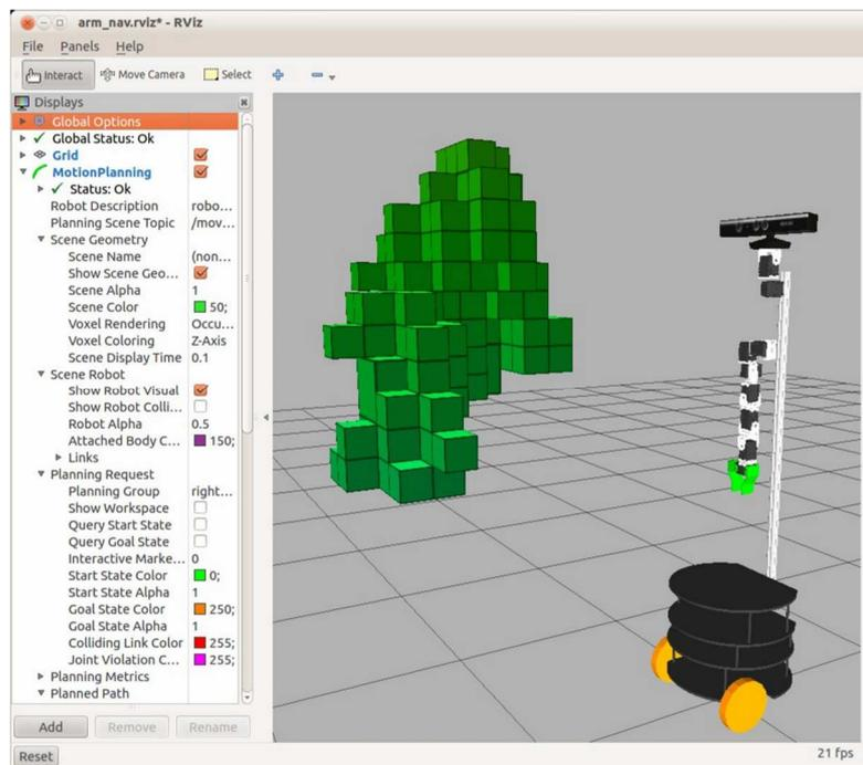
If you don't see the boxes representing the octomap occupancy grid, check in RViz under the **Motion Planning** display, then open the **Scene Geometry** settings and ensure that the checkbox labeled **Show Scene Geometry** is checked. If you move objects in front of the camera, the octomap boxes should update accordingly.
