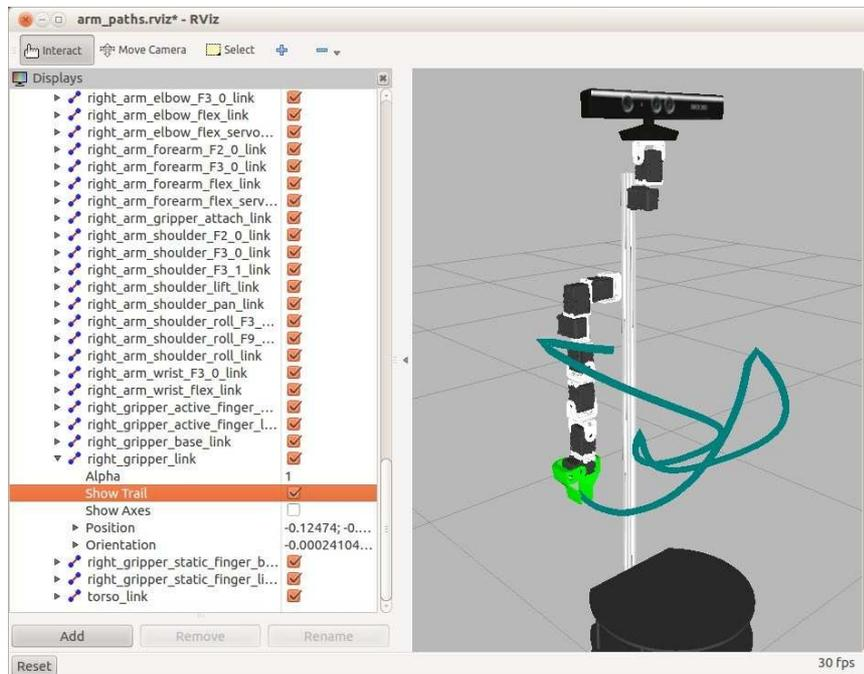
Notice that the all the trajectories are now curved. Note also that the gripper no longer stays horizontal along the triangular portion of the trajectory. What's more, if you run the command again, you will get a potentially different set of trajectories in between the same waypoints. This highlights another useful feature of the `compute_cartesian_path()` function: it can move the gripper the same way time after time.
