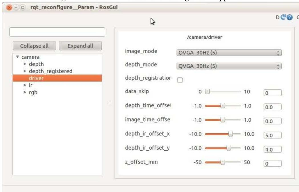
In the image above, we have clicked on the **camera** node and then selected the **driver** category. In the right-hand panel we can then change a number of the driver's parameters including the resolution using the pull-down menus labeled **image\_mode** and **depth\_mode**.
