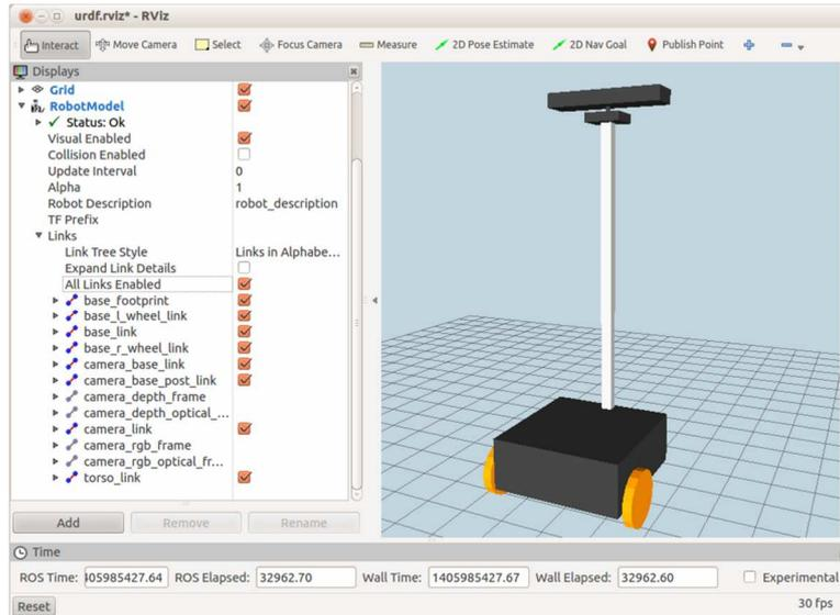
As you can see, we have modeled the Kinect using three pieces: a box for the base, a cylinder for the supporting post and another box for the camera body. Let's now look at the details.
