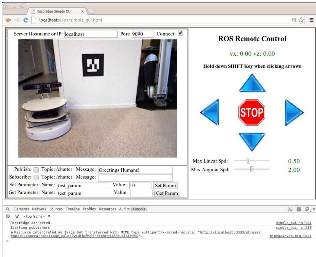
The lower panel displays the output of the Console. You can display messages here in your Javascript code using the `console.log()` command. In the screen shot above, our script displayed the two messages "Rosbridge connected" and "Starting publishers". Beside each message is the script name and line number that generated the output. You can click on the line number to go directly to the location in your script.
