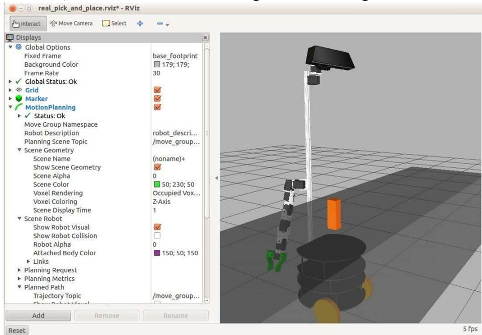
Here we see that the UBR-1 perception pipeline has successfully identified the table (shown in transparent gray) and the shape and location of the box sitting on top (shown in orange). Note that the box might sometimes appear as a cylinder rather than rectangular (and vice versa for cylindrical targets) since the fitting process is not perfect. For the most part, this will not affect grasping as long as the width of the virtual object is roughly the same in both cases.
