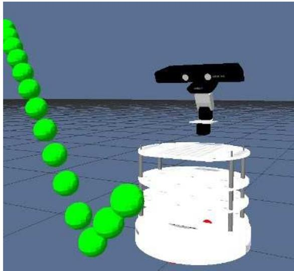
examples using the new head tracker. But first, let's create a node that publishes a fictional moving 3D point that we can use to test our tracking.
