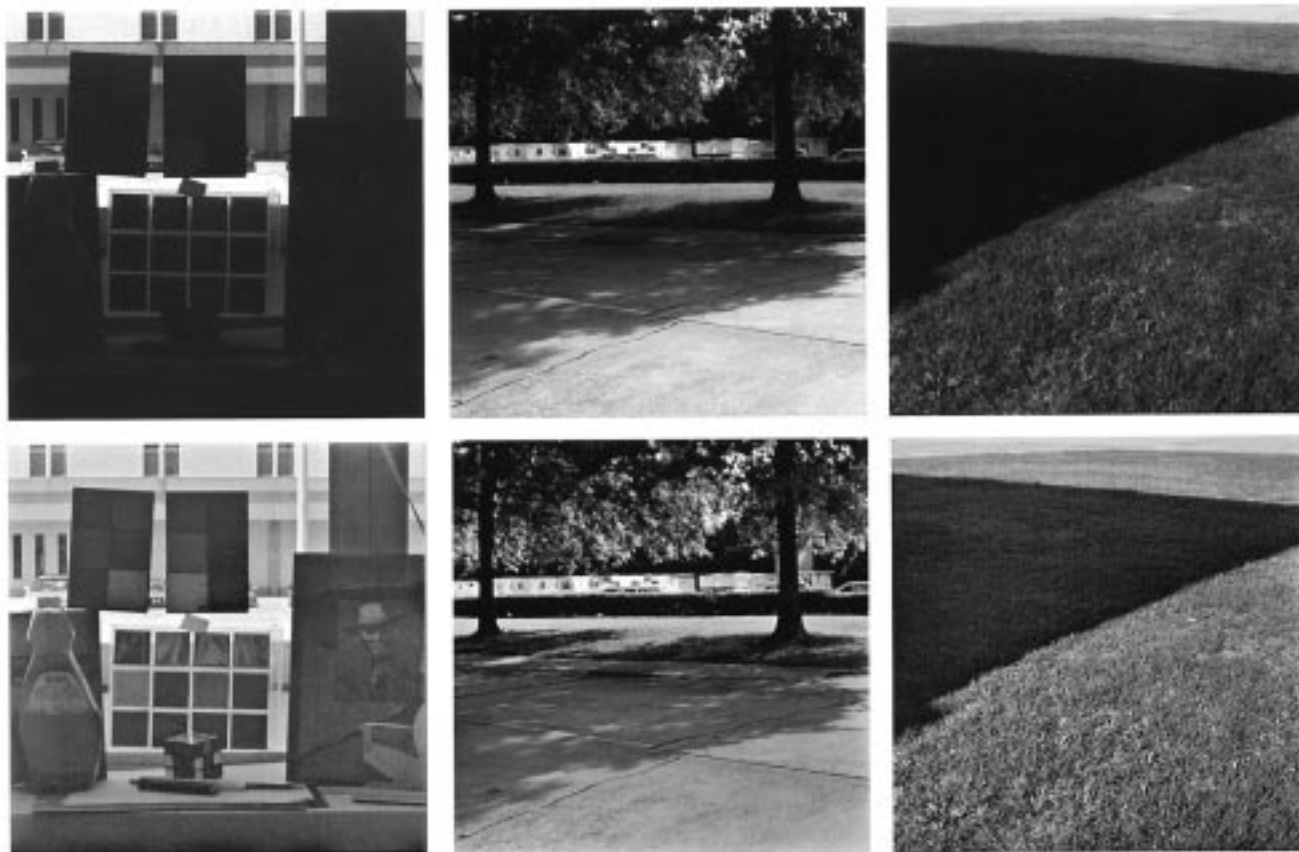
Fig. 3. Examples of test scenes processed with the multiscale retinex prior to color restoration. While color rendition of the left image is good, the other two are “grayed” to some extent. Dynamic range compression and tonal rendition are good for all and compare well with scene observation. Top row: Original. Bottom row: Multiscale retinex.
