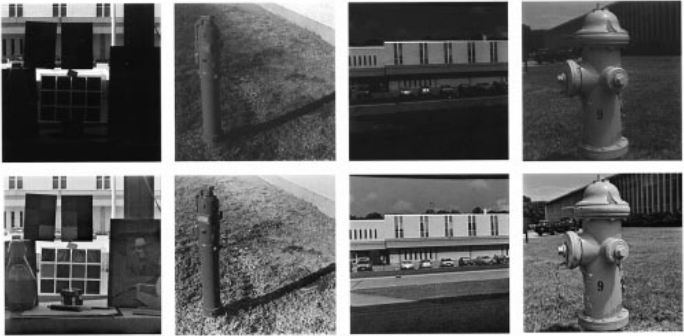
Fig. 5. Test scenes illustrating dynamic range compression, color, and tonal rendition, and automatic exposure correction. All processed images compare favorably with direct scene observation with the possible exception of leftmost image, which is even lighter and clearer for observation. This scene has the widest dynamic range and suggests that even stronger dynamic range compression may be needed for this case. Top row: Original. Bottom row: Multiscale retinex.
