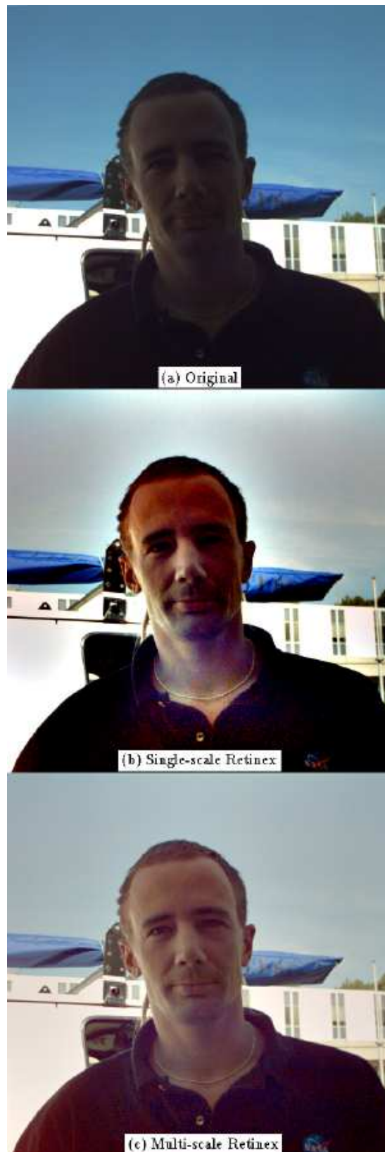
Figure 1: (a) Original (b) Single-scale Retinex (c) Multi-scale Retinex
